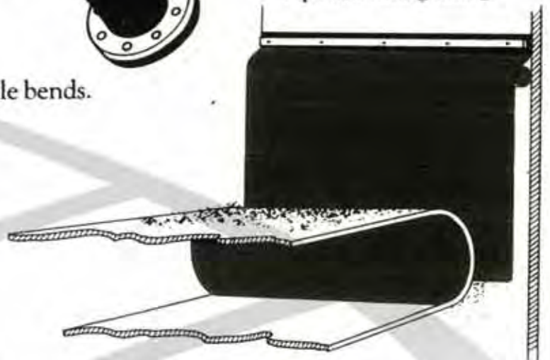
Pulley lagging and anti build up curtains.
